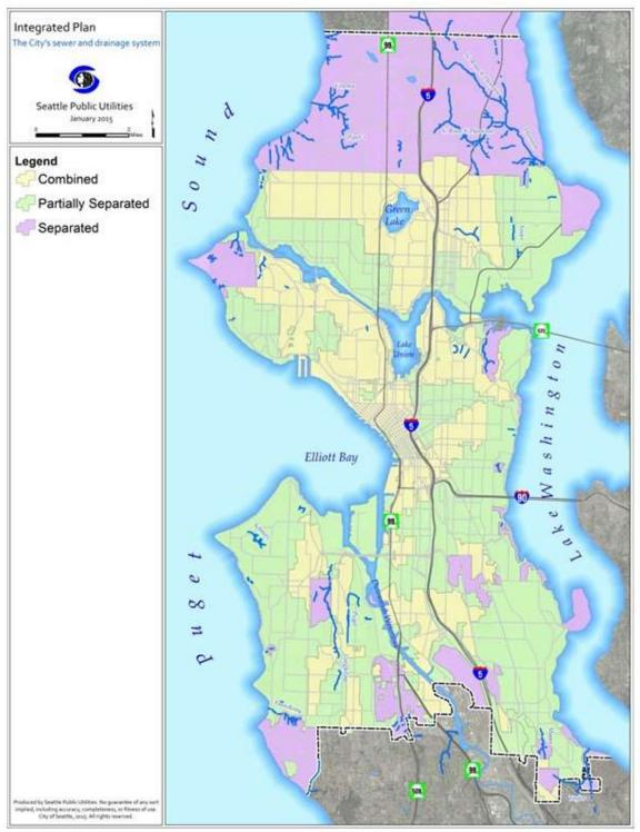
Figure I.1-1 The City of Seattle's Sewer and Drainage Systems
